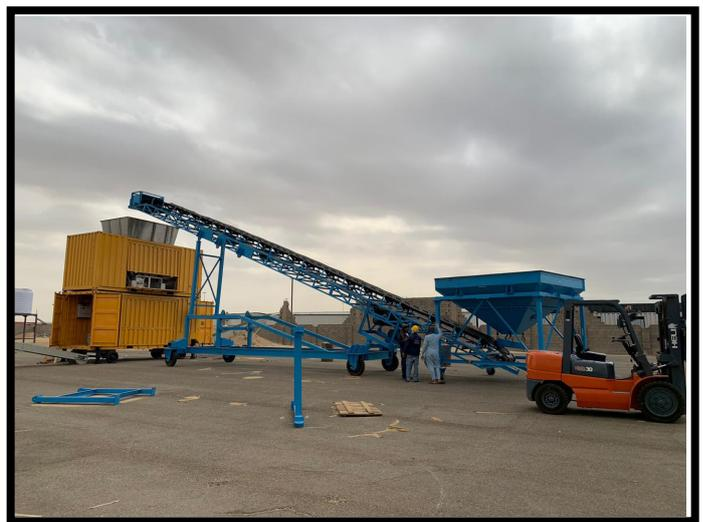
Belt conveyor system can transport materials in bulk and bagged, such as stone, sand, coal, concrete, cement, gravel, fertilizer, mineral ore, limestone, coke, sawdust, wood chip, bulk material, grain, corn flakes, carbon black, etc.
