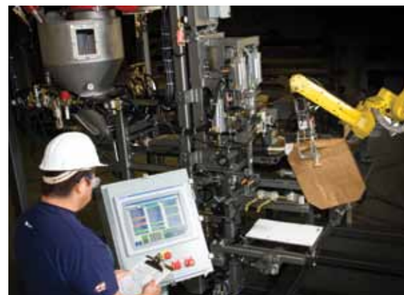
One single HMI controls scale, packer, sealer, and applicator
