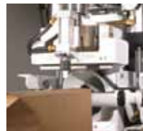
Bag is filled, then fill tube is purged of product and retracted from the spout of the bag.
