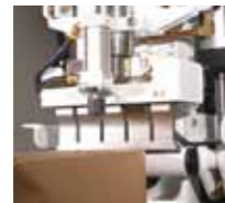
Bag valve is sealed and bag is discharged to a conveyor.
