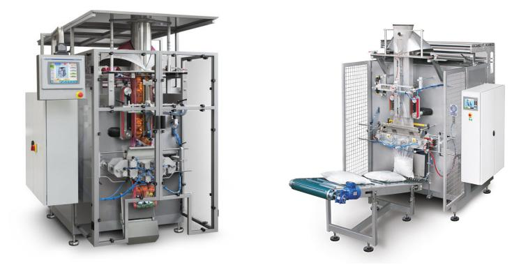
At Union Special Medway, we know that you cannot talk about bagging equipment without discussing vertical bagging systems. Vertical bagging systems essentially refer to a specific kind of vertical packaging machine also known as a vertical form fill seal machine. This particular piece of bagging machinery and equipment is a type of automatic packaging unit that is commonly used in the food packaging industry.
