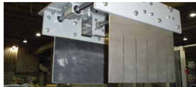
Bundle gripper with bundle height measuring system to compensate product density variations
