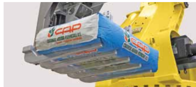
Special finger gripper with bag deposit by pusher
