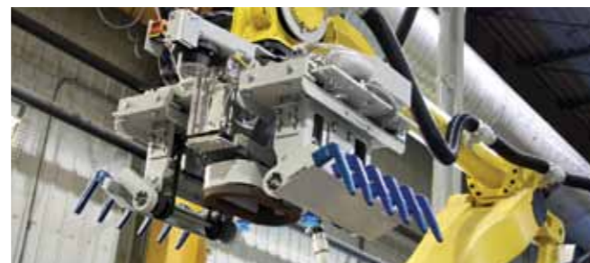
Dual function gripper: finger for palletizing and vacuum for depalletizing
