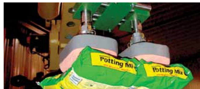
Vacuum gripper for bales, bags or boxes
