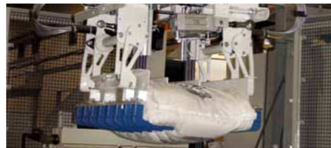
Finger gripper equipped with optional automatic bag width adjustment system
